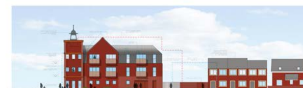
2018 Planning Design (large gable as per chapel, square tower with retained bell, roof form steps down)
